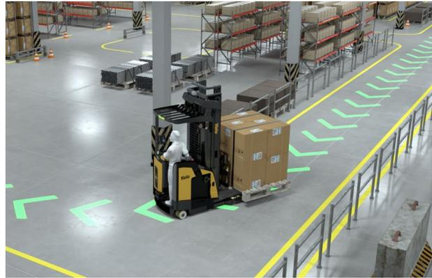
*Automatic speed reduction when cornering for stability*
