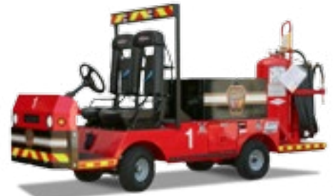
Bigfoot with SBCA seats, rear platform holds two Amerex units, battery roll-out box and light bar.
