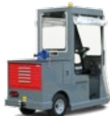
MX-600 mobile maintenance vehicle with cab, clear vinyl enclosure and strobe light.
