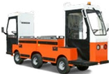
Double-ender drives forward only from either end in between rail cars.
