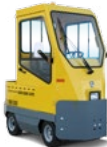
C-426AC tow tractor with cab, heavy duty front push plate and strobe light.
